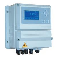
The NEP9000 and NEP9500 series are readiliy interfacable to the ANALITE TM5 Indicator/Controller unit the probe output must be either ±2.5V or 4-20mA. The ANALITE TM5 is ideal for industrial control and alarm applications. The ANALITE TM5 allows for the selection of wiping intervals as well as allowing field calibration.
