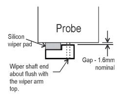
**NOTE:** It is imperrative that the set screw be fastened squarely aligned onto the flat on the shaft otherwise proper operation will be affected.
