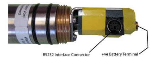
Connect the mating connector of the NEP495-CBL cable assembly provided to this connector.
