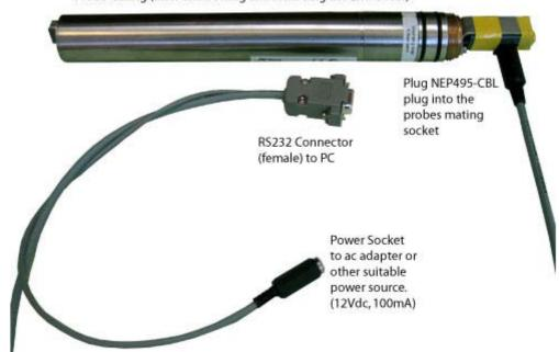
Probe Casing (after unscrewing and removing the End Cover)
