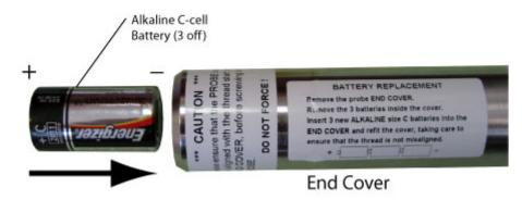
Remove any installed batteries by simply tipping them out. Place in the three new C-cells in the end cover with the negative terminals entering the tube first. Make sure the first battery makes contact with the contact spring at the end of the end cover. Ensure the subsequent batteries make contact with the previously inserted battery.
