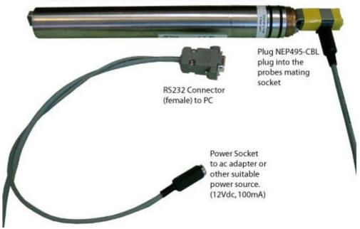
The probe must be externally powered during configuration or data download. Connect a suitable 12Vdc source to the power socket on the NEP495-CBL cable provided. The centre pin of this socket is negative polarity (-12Vdc).
