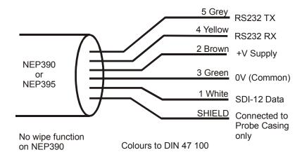
Ensure the RS232TX and RS232RX conductors are also individually insulated when operating in SDI-12 mode and likewise ensure the SDI-12 Data conductor is insulated when connected in RS232 mode.
