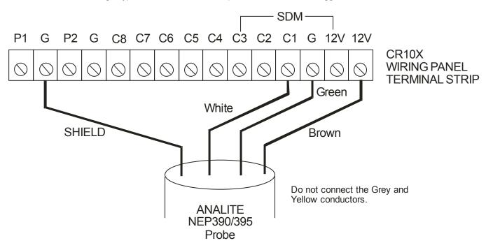
The logger will supply the necessary power for the ANALITE 390 or 395 probe.
