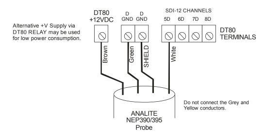
The logger will supply the necessary power for the ANALITE 390 or 395 probe.
