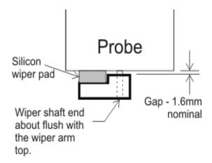
CAUTION: Do not over-tighten the set screw or manually attempt to rotate the wiper arm once set onto the shaft.
