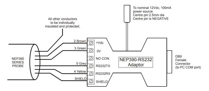
The adaptor requires power from an external 12Vdc power source. This powers the probe only and is in no way connected to the DB9 connector. The DB9 connector end of the adaptor is plugged into a PC COM port (also called the serial or RS232 port). A specification of an ac adapter that is suitable is near the back of this manual.
