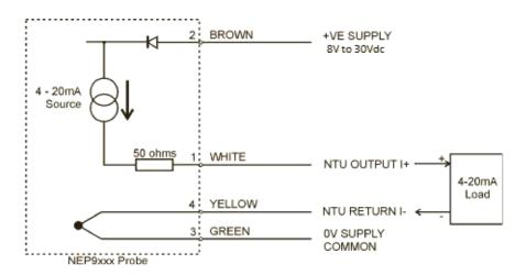
For very long cable runs (>200m), it may be advisable to connect the "NTU return" conductor to the "Supply Common" conductor at the end of the cable to reduce the voltage drop along the run. When a NEP-9500 series probe is ordered with the 4-20mA current output, the probe is configured as a (high) current source. The load must be less than 270 Ohms to ensure proper operation over the probe's specified power supply range.
