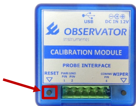
Figure 9.H: Calibration module “RESET”
