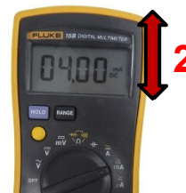
Figure 7.O: Scaling and calibrating 0NTU offset
