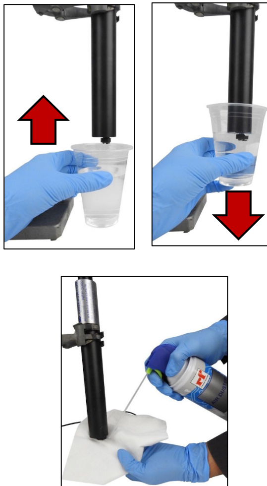
Figure 10.BB: Wash and dry the sensor
