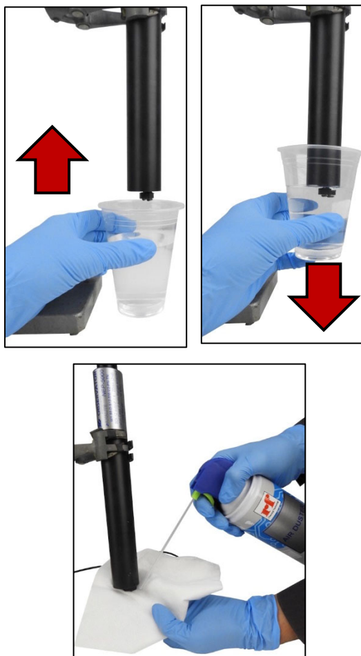
Figure 10.RR: Wash and dry the sensor
