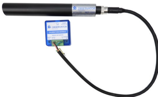
Figure 6.E: Example of configuration for SubConn SDI-12 probes
