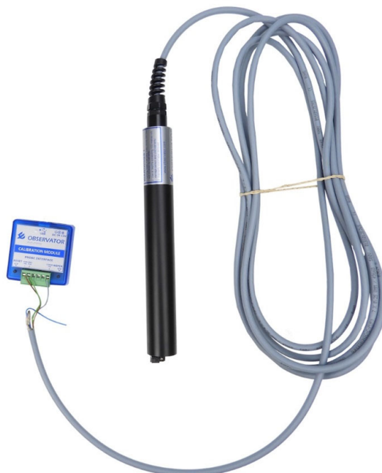
Figure 6.F: Example of configuration for SubConn SDI-12 probes
