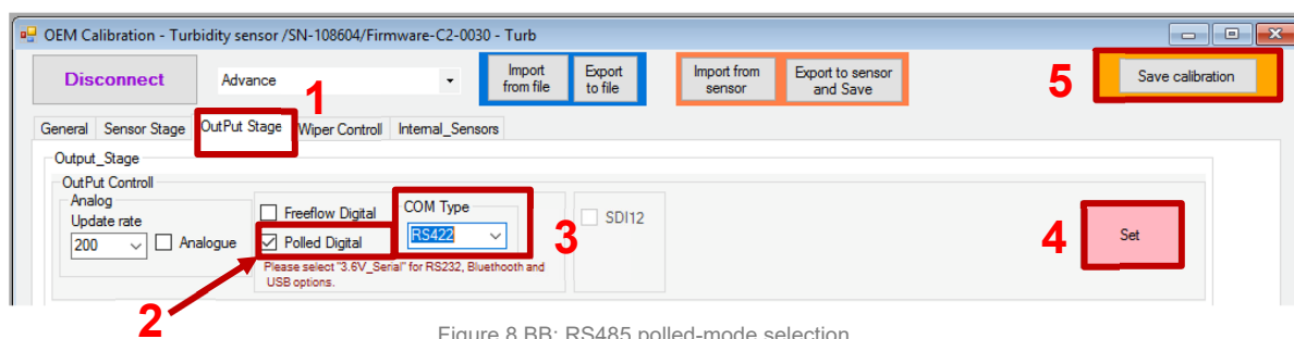
Figure 8.BB: RS485 polled-mode selection
