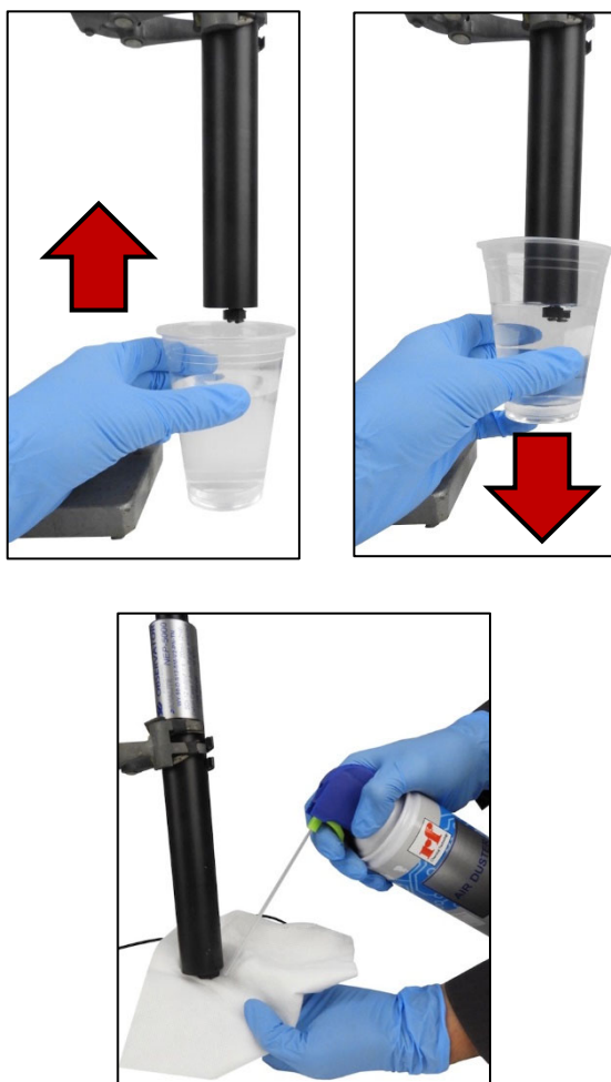
Figure 10.JJ: Wash and dry the sensor
