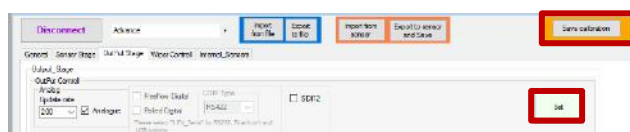
Figure 7.M: Set and save Analog current driver calibration
