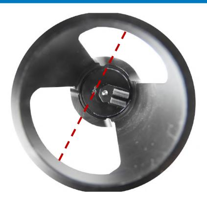
6. Use a grub screw driver and tighten the three screws to seal the shroud to the probe.
