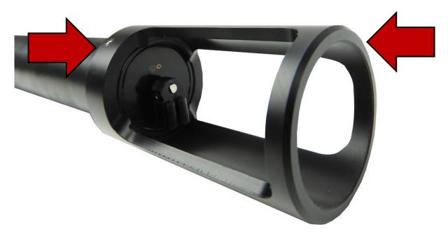
4. If you purchased the shroud at the same time as the probe, the probe will be marked with a "dot" to facilitate the installation. Line up the shroud indicator with the probe indicator.
